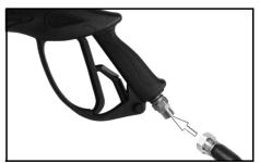
Connect the spray lance to the gun assembly and tighten securely by turning the locking ring.
